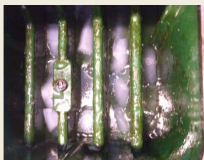
Figure 1: Blocks of gelled Solvitose® Greenmelt in the tank at 95°C (left initial, middle after 3 minutes, right after 8 minutes). Optimal settings depend on the dry solid content of Solvitose® Greenmelt. In this study we evaluated a solution with 53% and 55% refraction. With the following settings: Tank 95°C, Hose 97°C, Jetting head 98°C, Adhesive pressure 4 bar (53%) or 3 bar (55%), Jetting head type: SX Diamond, needle nozzle an excellent application and run ability was achieved.
