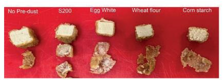
The picture clearly shows that only potato protein and egg white make the coating stick to the plant-based meat substrate, the other coatings can easily be peeled off.
